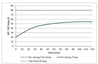
Tested @ ambient temp of 70F (21.1C) @ max run pressure
