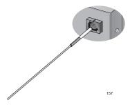
Figure 32. Cleaning a Recessed Ferrule
