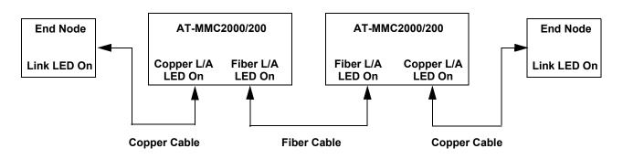
Figure 6. SML in Normal Condition with Two Media Converters
