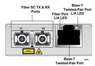
Figure 10. AT-MMC2000/200 Series nn/SC Front Panel
