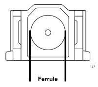
Figure 27. Ferrule in an SC Connector Plug
