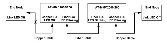
Figure 7. SML with Copper Connection to End Node Down
