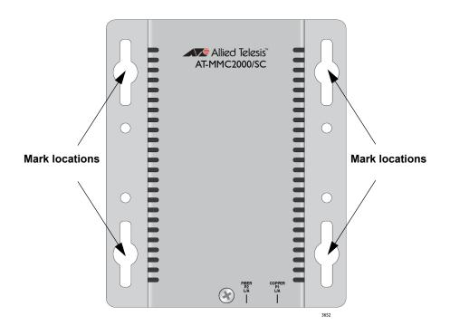
Figure 20. Marking the Screw Hole Locations
