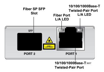
Figure 13. AT-MMC2000/SP Front Panel
