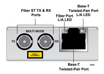
Figure 11. AT-MMC2000/200 Series nn/ST Front Panel
