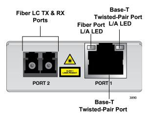
Figure 12. AT-MMC2000/200 Series *nn*/LC Front Panel
