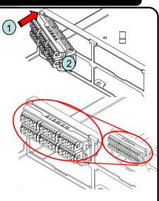
To remove the adapter plate, depress the latch on the right side of the plate and rotate toward the left. The plate can then be removed from the panel.
