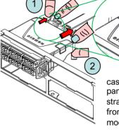
To remove the module or cassette from the rear of the panel, pull the release tether straight back to disengage from the panel and pull the module free.
