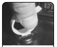
Install two fiber management clips in front of enclosure by inserting into appropriate holes and turning 45 degrees to lock into place (clip opening should face forward).
