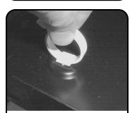
Install four fiber management clips in the rear of the enclosure by inserting into appropriate holes and turning 45 degrees to lock into place (clip opening should face the outer walls of the enclosure).
