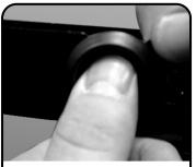
For dust proofing - Install feed-through grommet into un-used access hole as shown.
