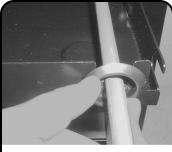
Slide a grommet onto the incoming cable and, to enable sufficient cable slack, push the grommet back one meter (3.28 ft) from the cut end of the cable. Install grommet into desired cable access hole.
