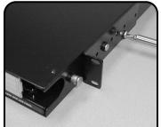
The enclosure can be mounted so that the protrusion from the front of the rack is either 51mm (2 in.) or 102mm (4 in.). Align the mounting bracket holes with the appropriate holes in the enclosure and secure a mounting bracket to each side of the enclosure using the two screws and plastic washers provided.
