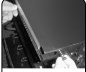
To slide tray out the front, grip the head of the front spring-loaded latch (located on the right side of enclosure) and pull out. While head is held in the out (un-locked) position, grasp knob at front of tray and pull towards you until first stop.
