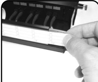
**16** Return label bracket into position at front of tray. Mark ports IDs on the labels provided and then insert the labels into the appropriate holder on the label bracket.
