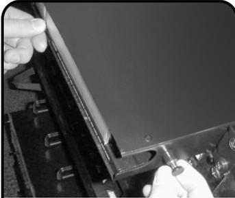
**3** To slide tray out the front, grip the head of the front spring-loaded latch (located on the right side of enclosure) and pull out. While head is held in the out (un-locked) position, grasp knob at front of tray and pull towards you until first stop.
