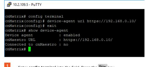
Enter config terminal into the field. Press the Enter key.
