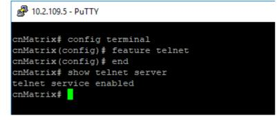
Enter **config terminal** into the field. Press the **Enter** key.
