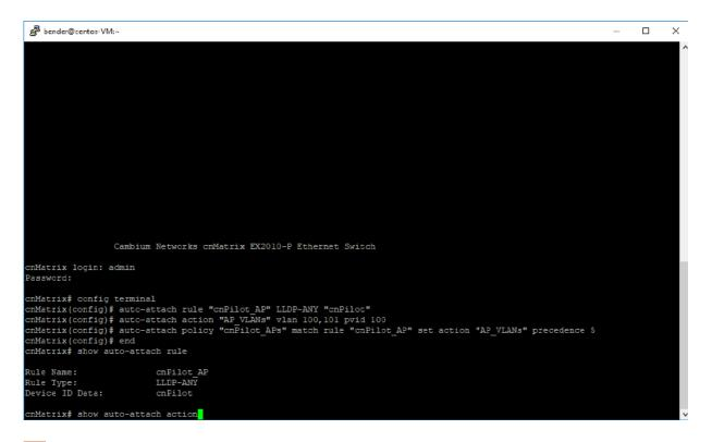
Enter **show auto-attach action** into the field to display Auto-Attach action information. Press the **Enter** key.
