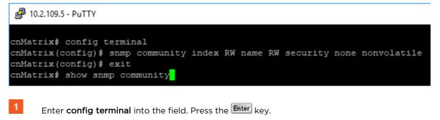
2 Enter snmp community index RW name RW security none nonvolatile into the field to configure the SNMP community details. Press the Enter key.
