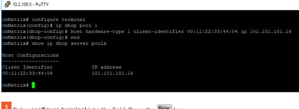
Enter **configure terminal** into the field. Press the **Enter** key.
