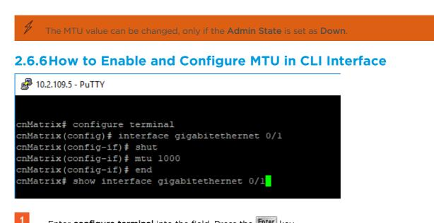
Enter **configure terminal** into the field. Press the **Enter** key.
