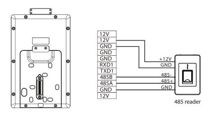
**Note:** 485A and 485B can be connected to the barrier gate or the 485 reader, but cannot be connected to the gate and the reader at the same time.
