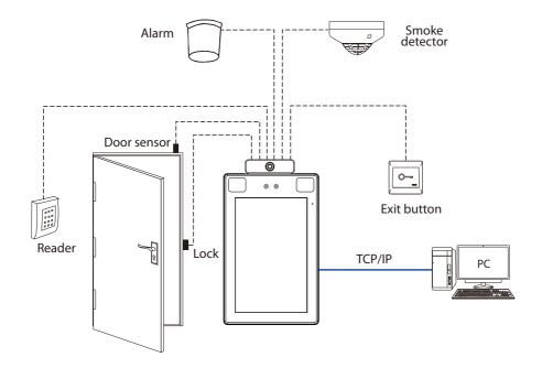
7 Door Sensor, Exit Button & Alarm Connection
