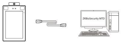
Default IP address: 192.168.1.201 Subnet mask: 255.255.255.0 IP address: 192.168.1.130 Subnet mask: 255.255.255.0
