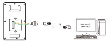
Default IP address: 192.168.1.201 Subnet mask: 255.255.255.0 IP address: 192.168.1.130 Subnet mask: 255.255.255.0
