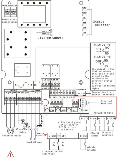
Cut off power before installation or repairation. Notice the difference between 110V and 220V voltage input.
