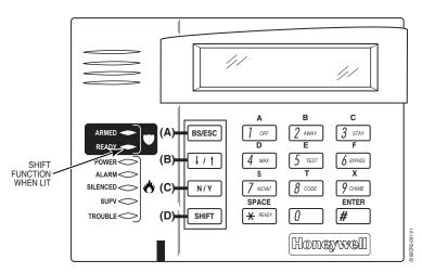
Figure 1: 6160CR-2 Key Functions for Programming the Communicator
