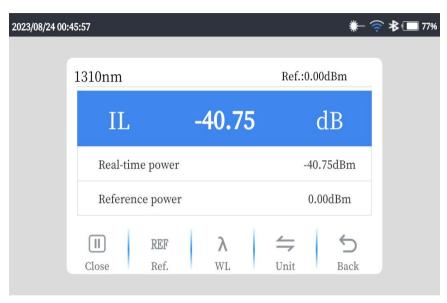
optical power meter OPM, and the IL displayed in real time is the insertion loss value.
