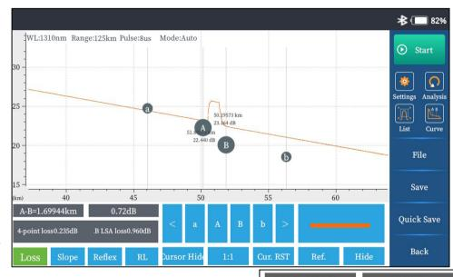
The 4-point method calculates the event loss in real time, and the LSA method calculates the A-B cursor loss in real time, as shown on the right below.
