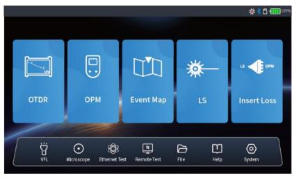
The quick operation interface controls the Bluetooth switch, Type-C USB (data transfer) switch, red light switch, quick screenshot, main sound switch, and brightness adjustment, and can also perform shortcut operations of shutting down and returning to the homepage.
