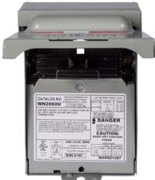
Siemens Low Voltage Residential Load Centers AC Disconnects - Siemens Pull Out ACD Non Fused Steel are Residential Enclosures AC Disconnects. Type: AC DISCONNECT Application: DISCONNECTING DEDICATED LOADS Standard: UL Voltage Rating: 240 V Amperage Rating: 60A Interrupt Rating: 10K Enclosure: NEMA 3R Mounting: SURFACE MOUNTING Size: 9.000X12.200X17.900
