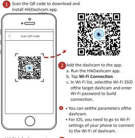
Dashcam Wi-Fi default parameters: 😗 Editthe dashcam password to Wi-Fi SSID: HIKVISION-XXXX activate itto avoid abnormal (XXXX refers to the lastfour recording after connecting to Wicharacters of verification code.) • Wi-Fi password: 1234567890 (please edit password after logging in for the firsttime.)
