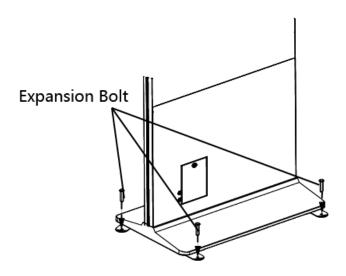
Figure 3-7 Secure the Screen
