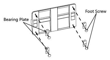
Figure 3-4 Mount Foot Screws
