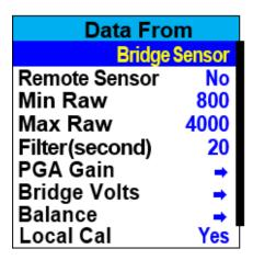
Figure 7-6 Data from Bridge Sensor Menu
