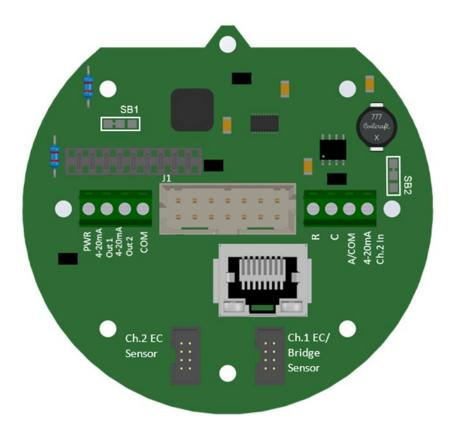
Figure 3-5 – TXP-T40 I/O Power Supply Board
