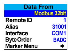
Figure 7-16 – Data from the Modbus 32-Bit Menu
