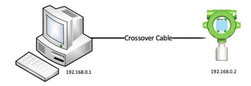
Figure 14-1 - Direct Connection with Crossover Cable
