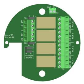
Figure 15-1 Relay / RS-485 Option Board
