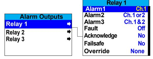
Figure 6-1 – Alarm Outputs Menu Tree
