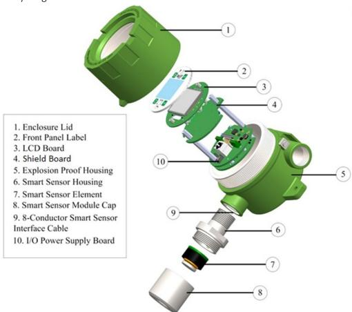
Figure 3-1 – Assembly Diagram
