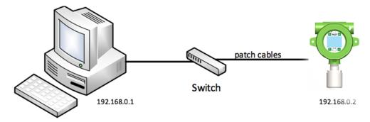
Figure 14-2 – Direct Connection with Switch and Patch Cables
