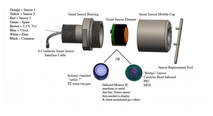
Figure 3-6 – Smart Sensor Head Assembly
