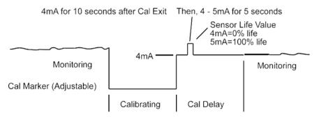
Figure 9-4 – Send SensrLife Time Diagram
