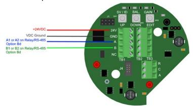
Figure 16-2 – Remote sensor Option Board Wiring
