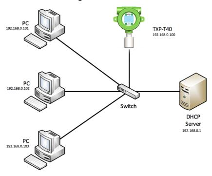
Figure 14-3 – Connecting the TXP-t40 to an Existing LAN
