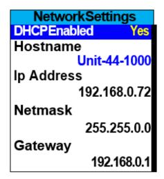
Figure 14-10 – Network Settings Menu with DHCP Enabled
