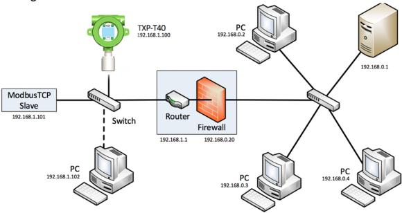
Figure 14-4 – Connecting the TXP-T40 to an Isolated Network
