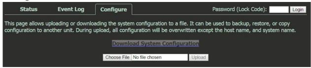
Figure 13-5 Config Transfer Screen
