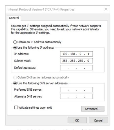
Figure 14-9 – Internet Protocol Version 4 (TCP/IPv4)
