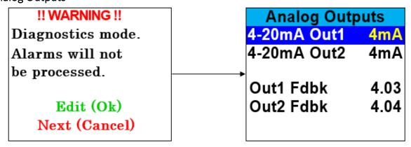
Figure 11-3 – Analog Outputs Diagnostics Menu
