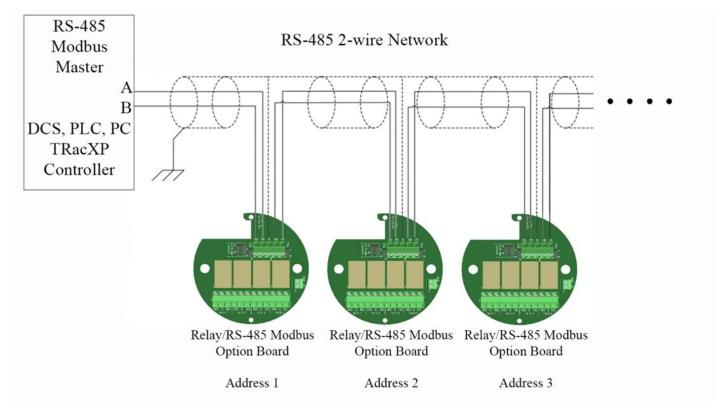
Figure 15-2 – RS-485 Modbus Wiring
