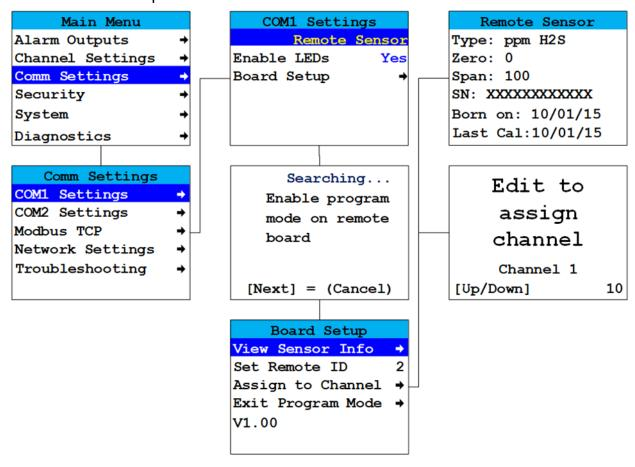
Figure 16-3 – Remote Sensor Setup Menus
