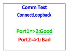
Figure 11-5 – Serial Ports Diagnostics Menu
