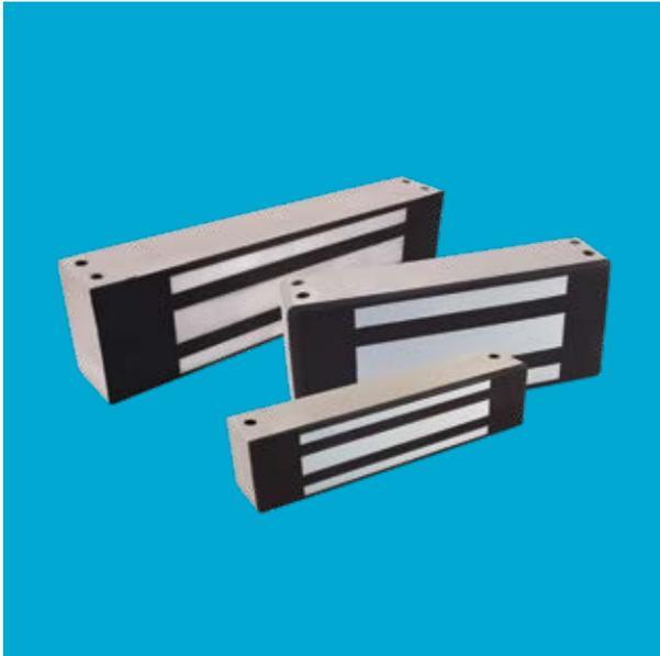
Electromagnetic locks (maglocks) can be installed on various frames and doors using accessories. To figure out what you need for a maglock install, first measure the door stop. Most maglocks require 2-1/4" to 2-1/2" of flat mounting space for direct mount or mounting bracket. You may need one or more accessories if the door stop is less than 2-1/2".
