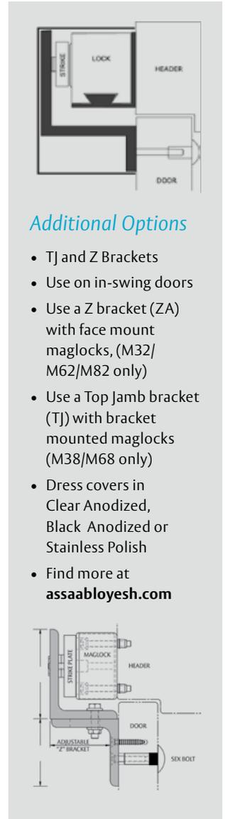
Accessories are available in a clear aluminum or black anodized finish. Verify length of magnetic lock before ordering mounting accessories.
