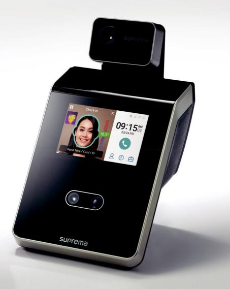
**Suprema FaceStation 2 with Temperature Detection** combines Suprema's face recognition terminal\* with Suprema Thermal Camera to detect users with elevated skin temperature.
