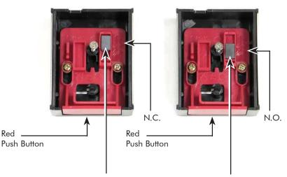
With SS-077 the magnet is in the UP (N.C.) position.
