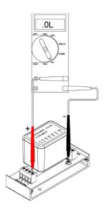
The DTK-2MHLP Series utilizes a multi-stage hybrid circuit design that incorporates SAD (Silicon Avalanche Diode) technology and a Slo-Blo (Fuse). This device is passive to the circuit until there is a change in voltage (overvoltage). Then, the component turns on and shorts the overvoltage energy down the ground path and away from the circuit. After the fault is removed, the components release their hold on ground; they reset and get ready for the next event.
