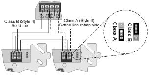
Figure 1: SLC Wiring
