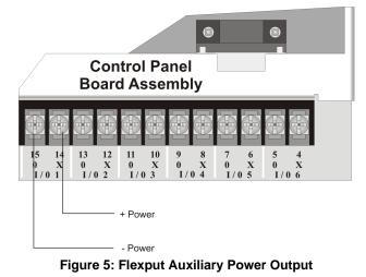
2. Configure the auxiliary power output for constant output through programming. Refer to the FACP installation manual form more information.
