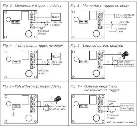
Note: regarding DIP switch #1: Sometimes DIP switch #1 will function as an instant/delay control, but when it is ON, its actual function depends on how DIP switch #3 is set.
