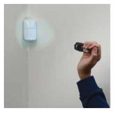
**Snap Walk Test:** Triggers walk test mode with the flick of a flashlight, reducing the number of trips to the sensor during installation.
