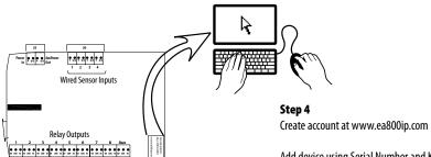
Add device using Serial Number and Key Code shown on the Ethernet jack. Configure device and sensors.
