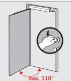
**6** Following the learning cycle, the PORTEO door assistant is ready for operation. Now you can perform further adjustments like speed, hold-open time or adjustments regarding the optional accessories like for example the electric strike, see adjustments page 22 and 23.
