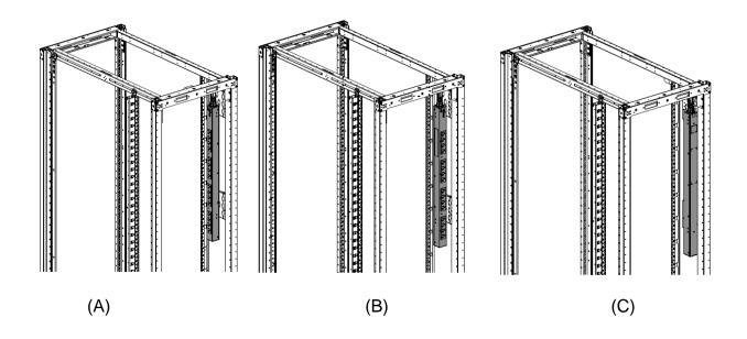
**NOTE:** The above installation methods are true for all vertical models except for the high-density models. Those units can only mount on its side with outlets facing the back of the rack. Reference the high density PDU installation section for installation instructions.
