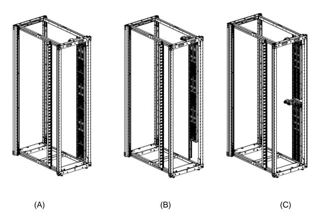
**NOTE:** (A) Two full-height PDUs with outlets facing in towards the center of the rack; (B) Two mid-height PDUs with outlets facing in towards center of the rack; (C) Four half-height PDUs with outlets facing in towards center of the rack.
