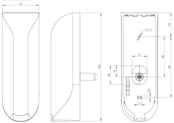
Figure 1: NVITE reader dimensions (mm)
