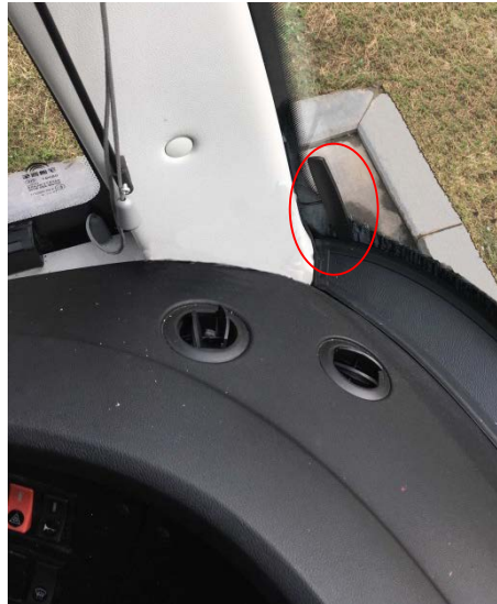
Figure 2-18 Inside installation of mobile network antenna
