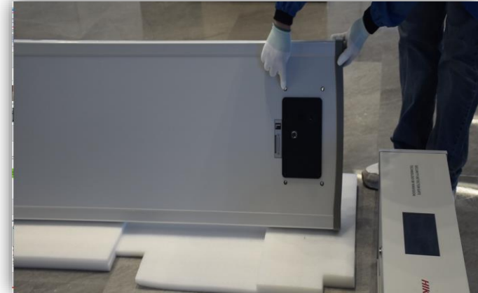
3. Left side panel → left side of main box Right side panel → right side of main box
