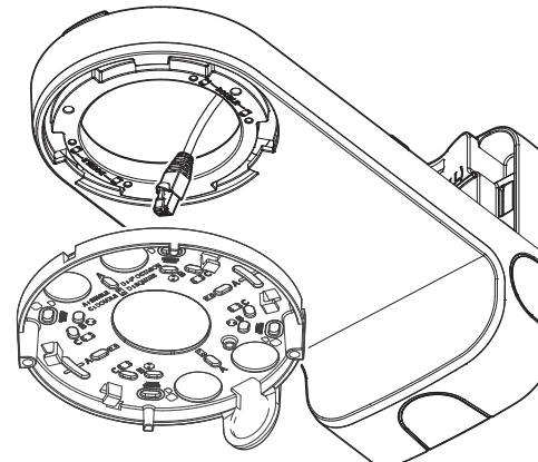
❖ If installed on a pole, conduit installation is only possible at the bottom.
