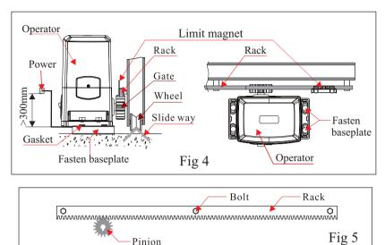
2.2.2 Install the limit magnet at proper position on the steel rack.
