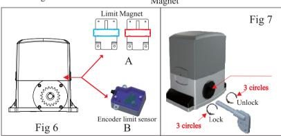
Move the gate manually to the open limit and close limit,mark the points on the rack,then,fix the limit magnets at the limit points on the rack,
