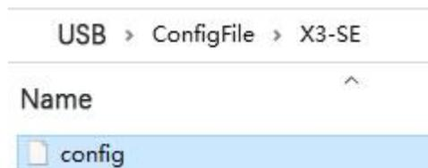
Connect the USB flash drive containing the config file to another device, select "Import", and the device will prompt that the parameter import is successful. Parameters in the config file contained in the USB flash drive will be imported into the device (registration information such as license plate number will not be imported).
