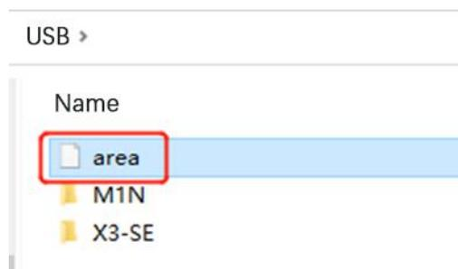
Import: Place the Geo-fence file in the root directory of a USB flash drive and tap Import to import the file. (It can also be issued remotely via the CEIBA platform.)
