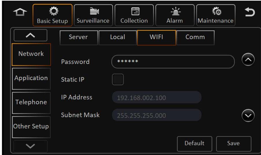
For WIFI network, you can obtain the IP address automatically, and also can configure it with a static IP.
