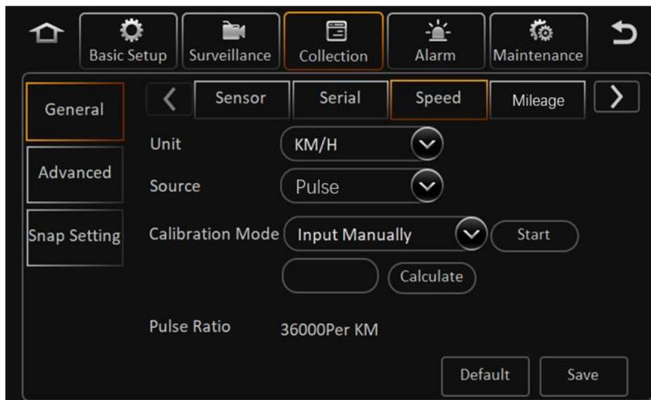
The pulse speed calibration function is to obtain the value of the pulse coefficient. The pulse coefficient is the number of pulses generated per kilometer of the vehicle.
