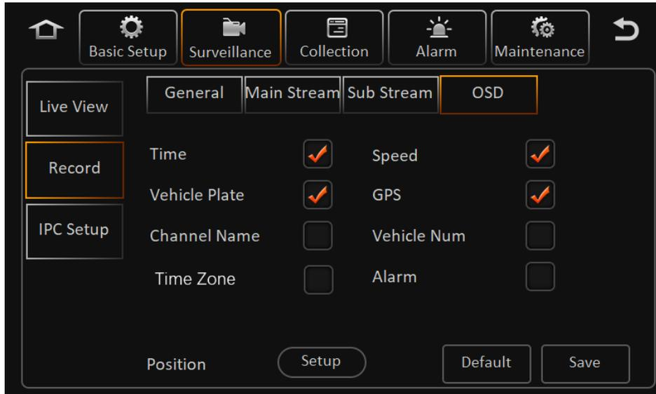
The OSD here is a recording function that allows you to superimpose selected information on the recording, and is different from OSD superimposition in live view preview.
