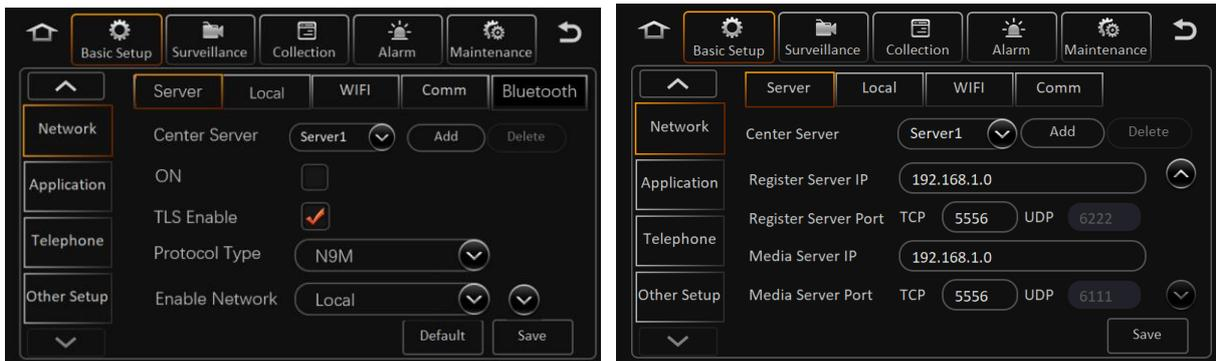
The device can connect to multiple servers at the same time according to the configuration. By default, one server is connected. It supports adding or deleting servers manually. Servers whose information can be reported include the CEIBA2 server, maintenance server, FT platform, and customer platform.
