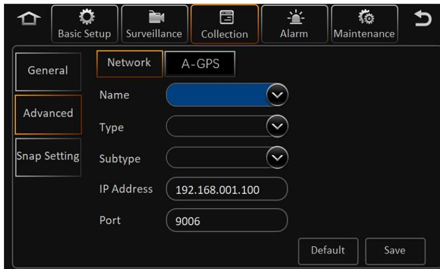
In addition, click **Login Avatar** > **Setup** > **Data Collection** > **Advanced** on the live view interface, A-GPS can also be set, as shown in the following figure:
