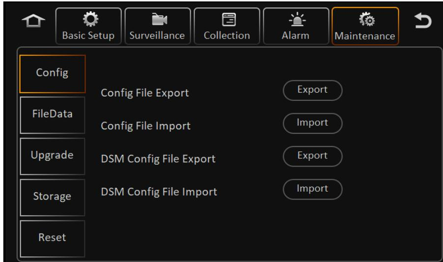
Connect the device to a USB flash drive, select the Export button in the Config File Export line to export the config file to the root directory of the USB flash drive, generating a folder named "ConfigFile". There is an MDVR model folder (such as X3-SE) in the ConfigFile. The MDVR model folder contains the parameter file named config. The config file contains all the parameters that can be exported from the MDVR (registration information such as license plate number will not be exported).
