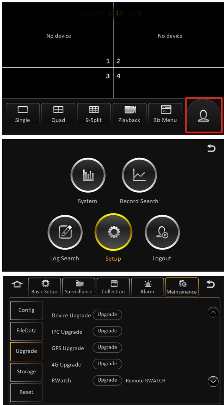
Create a folder named "upgrade" under the root directory of a USB flash drive, place the upgrade file in the folder, plug the USB flash drive into the USB port on the front panel of the MDVR, and tap the corresponding upgrade
