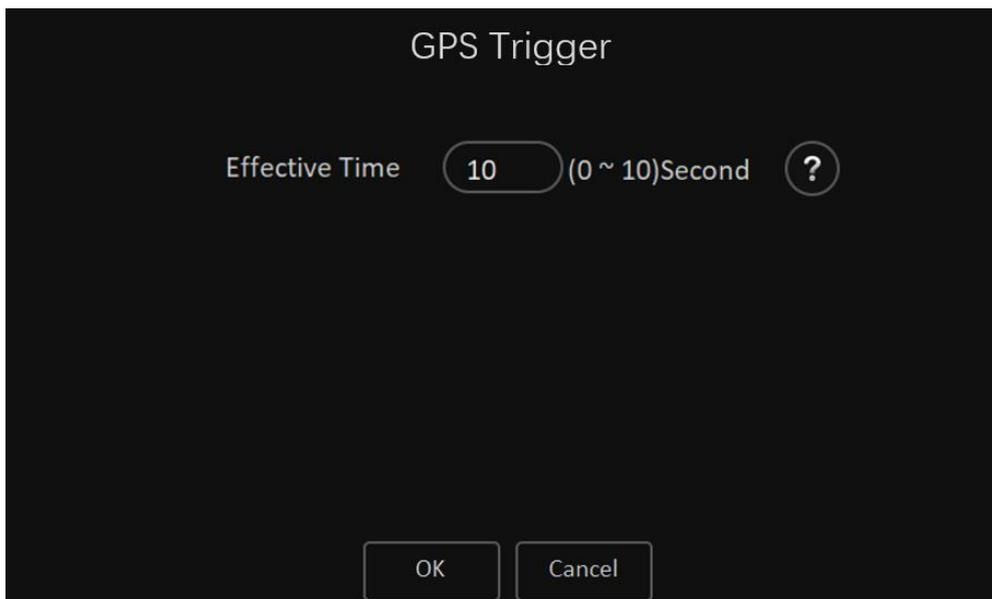
Effective Time : indicates a time period during which an alarm that is repeatedly triggered after being cleared will be considered as a single alarm. The detailed description is the same as those of the IO alarm. The effective time of GPS alarm can be any of 0 ~ 10s.
