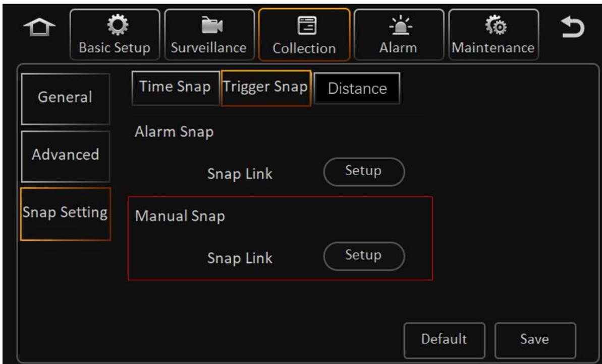
Tap Setup to enter the manual snap link screen, and please refer to Time Snap for the linkage. However, the manual snap does not have the Interval setup, it will take a snap picture once triggered.
