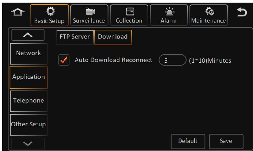
Tick to enable the Auto Download Reconnect and set the reconnection time between 1 and 10 min, the default is 5 min.
