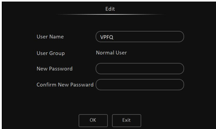
Enter the new User Name and Password, then after completion tap the "OK" button to return to the User Setup screen and tap the "Save" button.
