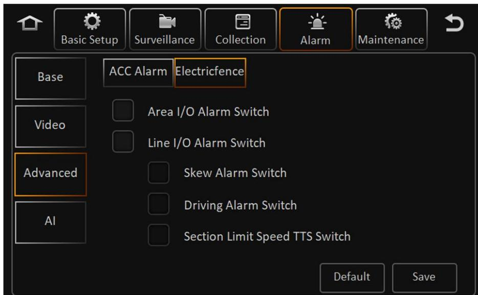
In this screen, you can only enable or disable the Geo-fence alarm and voice broadcast, and cannot set the location and range of the Geo-fence. The area and line of the Geo-fence can be set on the CEIBA platform.
