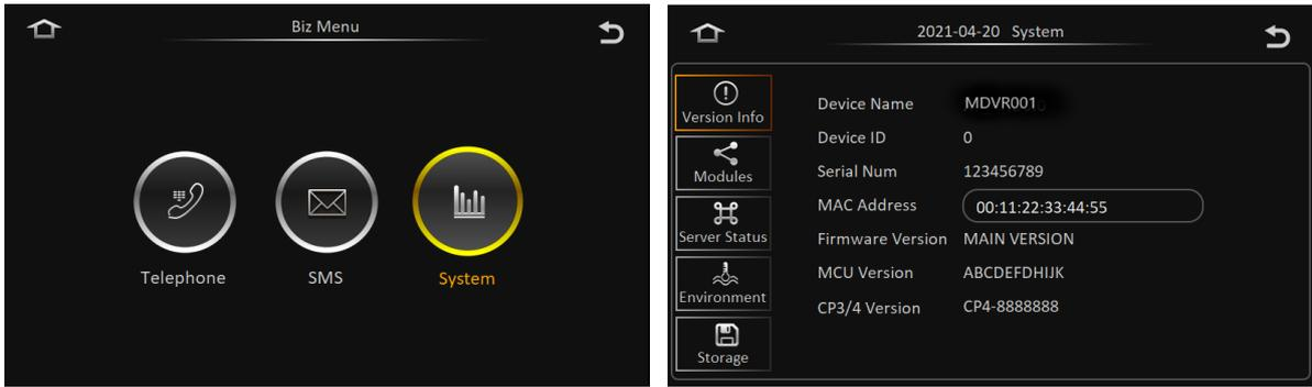
Version Info: displays Device Name, Device ID, Serial Num, MAC Address, Firmware Version, MCU Version, and CP4 Version. The MAC address can be modified. To do so, tap the input box and modify the address on the screen displayed, as shown in the following figure.
