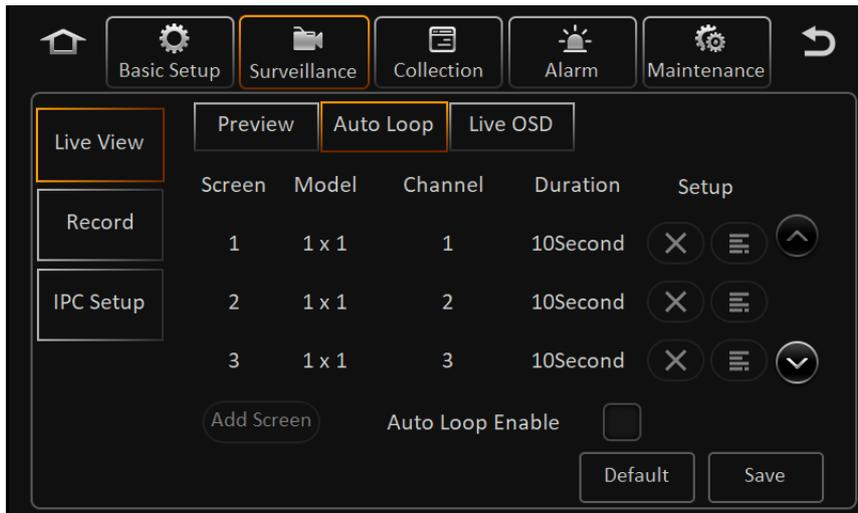
Below, you can enable the auto loop, delete and add the loop screen;
