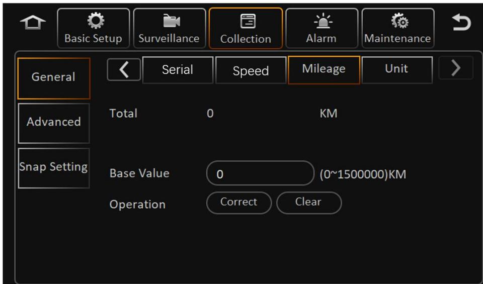
⚠ Note: The speed source of the mileage value is the same as the speed source selected by the vehicle speed, and no special source is required to set here.
