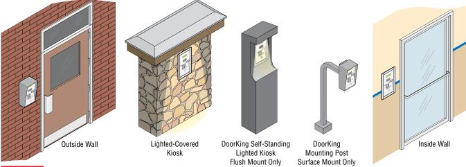
WARNING If this telephone entry system is used to control a vehicular gate with an automatic gate operator, the telephone entry system must be mounted a minimum of ten (10) feet away from the gate and gate operator, or in such a way that the user cannot come into contact with the gate or gate operator when using this entry system.
