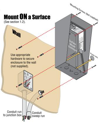
Examples of conduit runs that may be used, depending on how you choose to run the wiring. Some installations will allow the conduit to be run outside the wall and connect to the bottom of the enclosure but this is generally NOT recommended.
