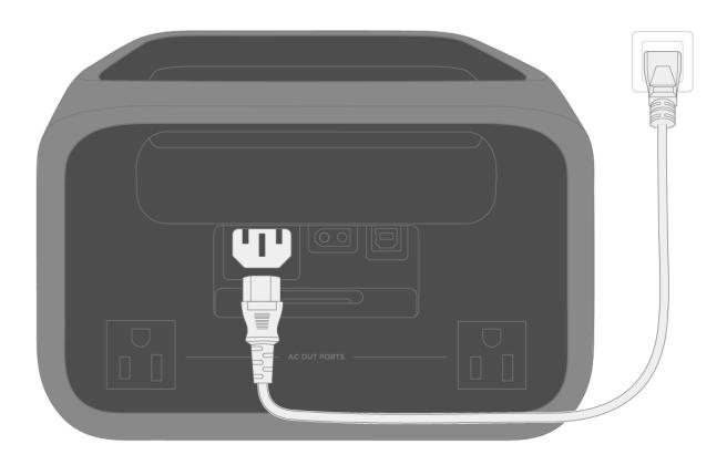
It's recommended that you use a power socket with a capacity of more than 10A and ensure that the working current of the socket is constantly greater than 10A.
