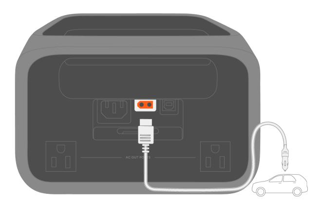
To avoid failure to start the vehicle due to insufficient car battery, start the vehicle first before you begin car charging. In addition, make sure that the car charging cable is securely connected to the cigarette lighter socket.
