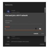
NOTE: If the WAVE-101 was previously in Access Point Mode prior to selecting Connect Mode, it will not scan for existing Wireless Access Points. The SSID/Password will have to be entered manually. To scan for available Wireless Access Points, change the mode to Disabled, press save, then select Connect mode.
