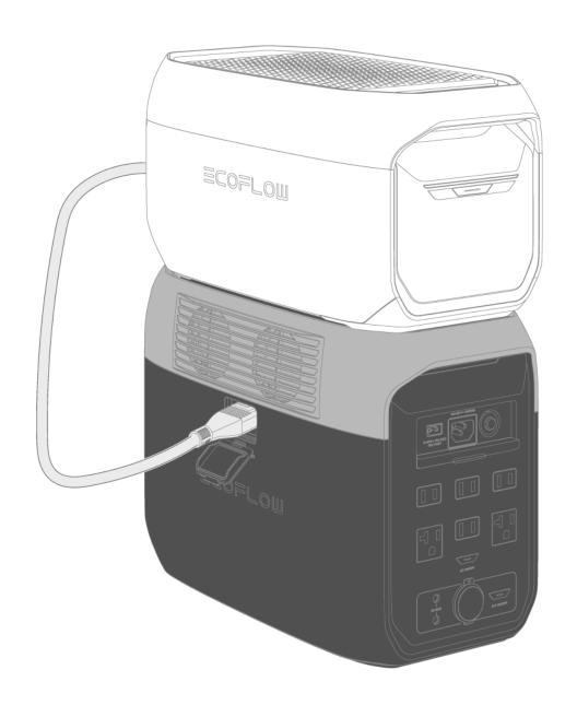
1. Connect the extra battery to the power station's Extra Battery port.
