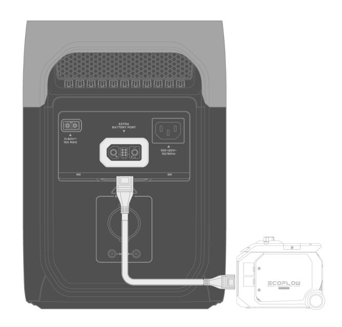
This connection method is only available via EcoFlow Smart Generators.
