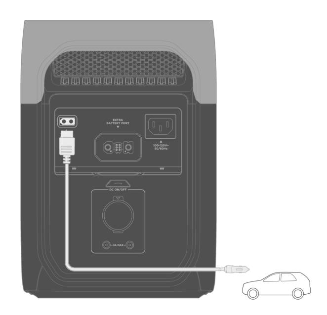
To avoid the start failure due to insufficient car battery, please connect the charging cable after the vehicle is started. In addition, please make sure that the cable is securely connected to the cigarette lighter.
