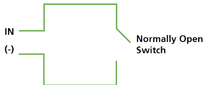
Figure 23: Normally Open Input Connection
