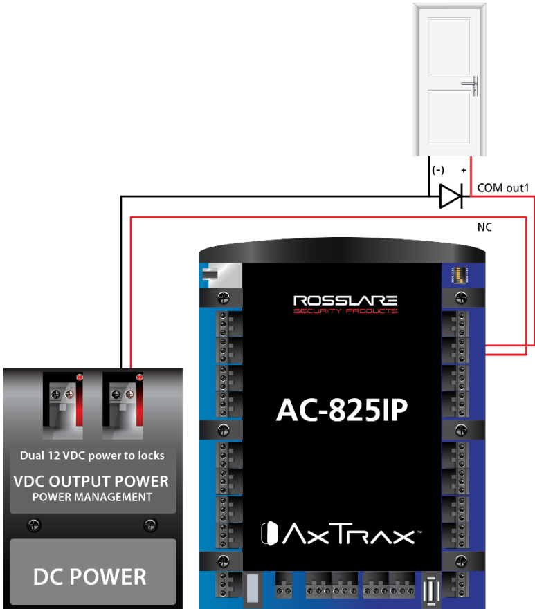
Figure 13: Door Lock – Failed Open
