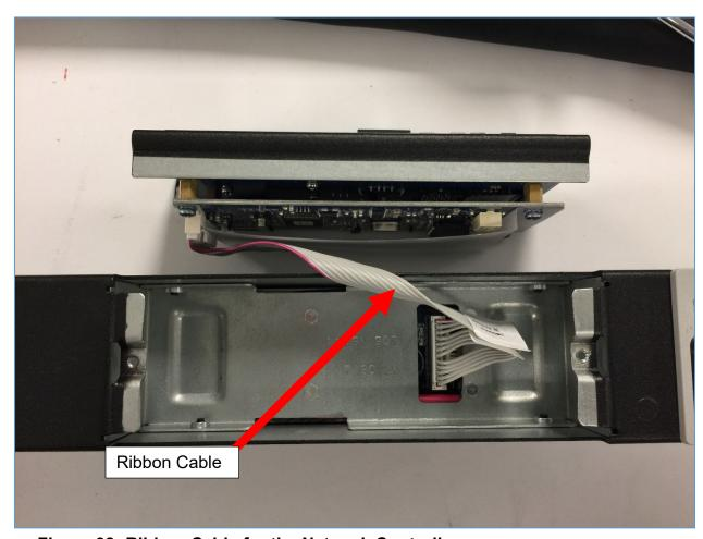
Figure 98: Ribbon Cable for the Network Controller
