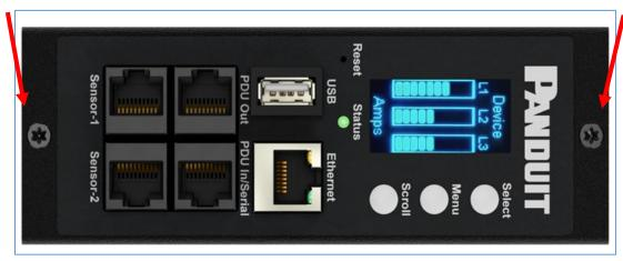
Figure 97: Screws on Network Controller
