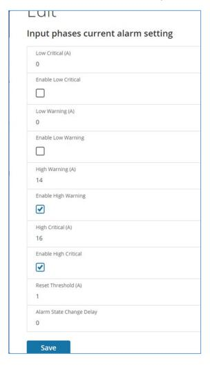
Figure 27: Phase Current Alarm
