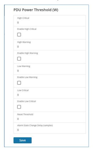
Figure 25: Power Threshold
