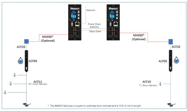
Figure 72: Connection Diagram for SmartZone Security Handle
