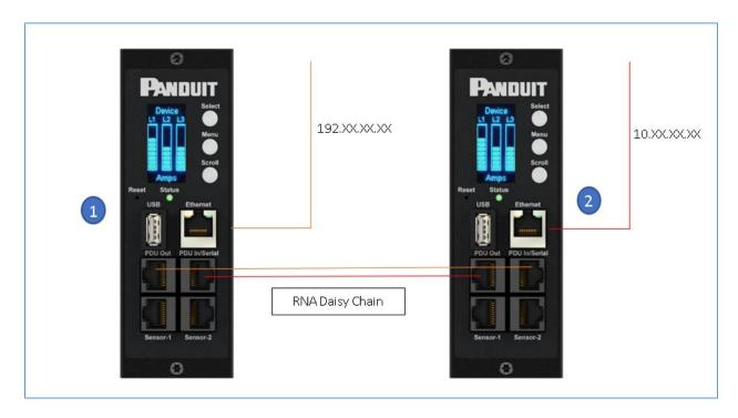
Figure 69: Connection Diagram RNA Daisy Chain
