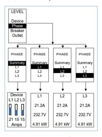
Figure 65: Phase Submenu
