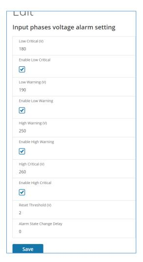
Figure 28: Phase Voltage Alarm
