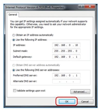
Figure 105: IP Settings for Direct Connection
