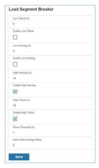
Figure 29: Load Segment Breaker
