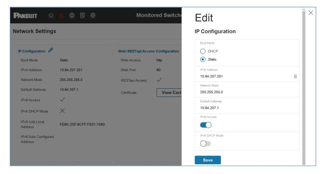
Web RESTapi Access Configuration can be used to set HTTP, HTTPS or Disable the onboard Web GUI.
