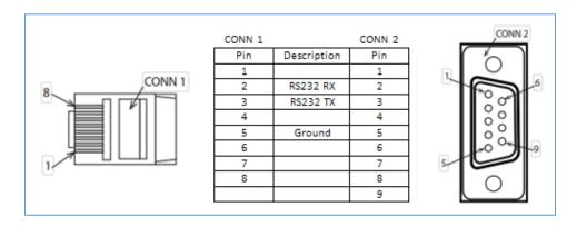
Figure 107: Serial Cable Pinout
