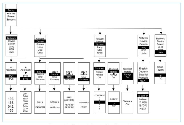
Figure 53: Network Controller Menu Structure
