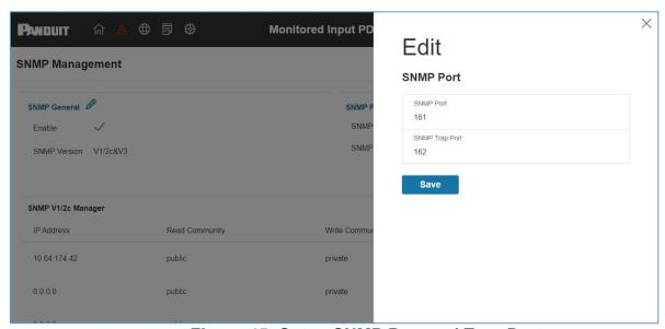
Figure 45: Setup SNMP Port and Trap Port
