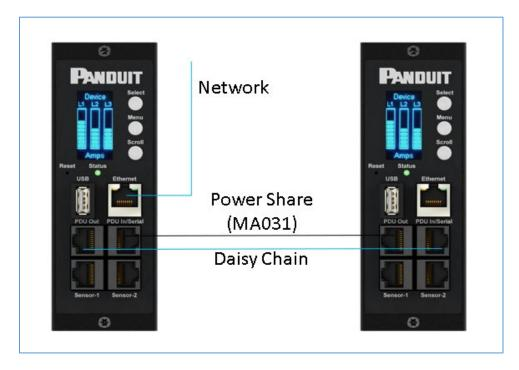
Figure 70: Connection Diagram Power Share & Daisy Chain
