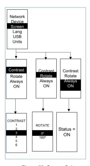
Figure 58: Screen Submenu
