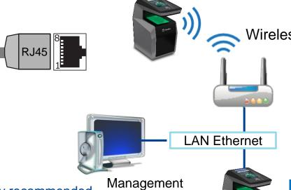
Use a category 6 shielding cable (120 Ohms) or better. It is strongly recommended to insert a repeater unit every 90 m.
