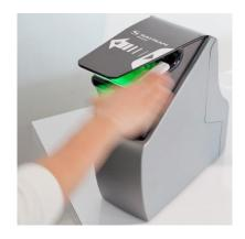
On Access Request, the terminal checks user's access rights using a biometric check. If the result of the check is successful (access granted), a message is sent to the Central Access Controller for additional access rights check.
