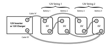
Fig. 3.7 Series-Parallel Connection
