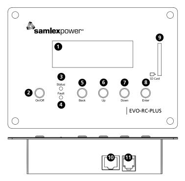
Fig 2.4(a) Optional Remote Control EVO-RC-PLUS
