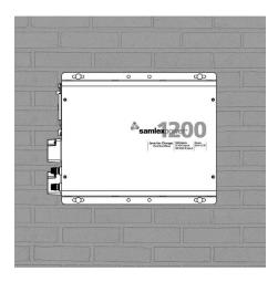
Fig 3.3 Mounting Arrangement 2: On Vertical Surface
