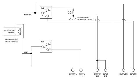
Fig 4.1 Operation of Transfer Relay and Neutral to Ground Bond Switching
