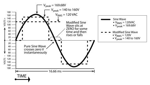
Fig 1.1 Pure and Modified Sine Waveforms for 120V, 60 Hz
