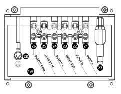
Fig 3.9.2(a) Pocket for AC Input and Output Connections for EVO-1212F-HW and EVO1224F-HW
