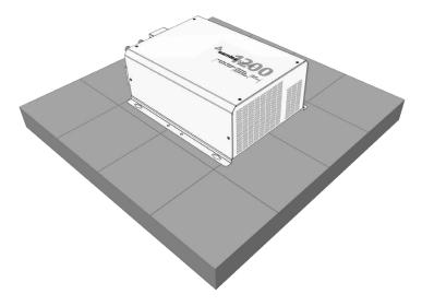
Fig 3.2 Mounting Arrangement No.1: Horizontally On Horizontal Surface
