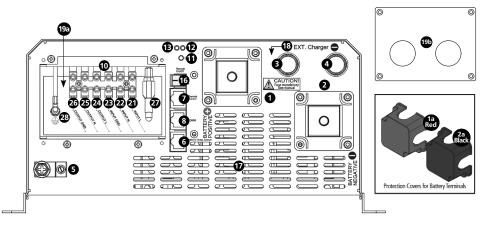
Fig 2.3 Hardwired AC Input and output connections: EVO-1212F-HW and EVO-1224F-HW
