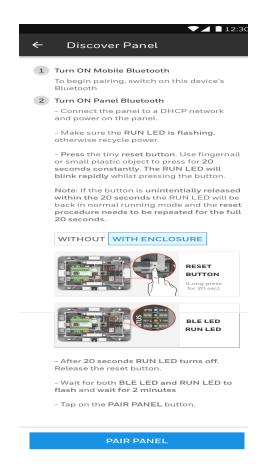
2. After the reset procedure, the BLE LED on the panel starts blinking. The RUN LED must blink slowly as well. This indicates the panel is ready to pair and send information about the panel
