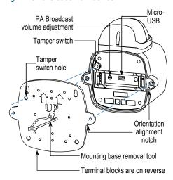
Fig. 2 Mounting base – inner side
