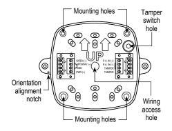
Fig. 3 Mounting base – terminal block detail
