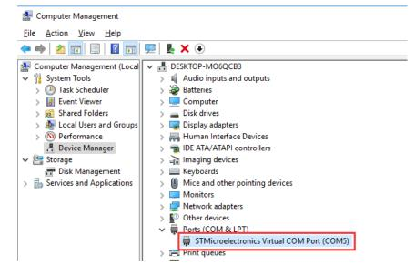
Note: After the driver installation is finished, if the preceding figure is not displayed, copy the **mdmcpq.inf** file to the **C:/windows/inf/** directory and **usbser.sys** file to the **C:/windows/system32/drivers/** directory, and then restart the computer.
