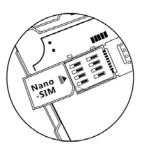
Insert the Nano-SIM into the card slot and close the back cover.
