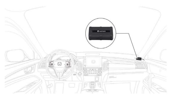
Mount the device in the vehicle by a cable tie or 3M double-sided tape.
