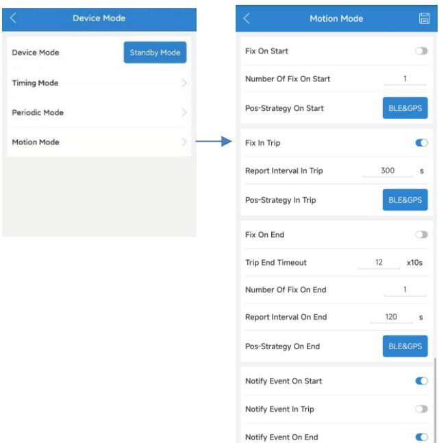
**Fix on start:** Whether the beginning of the movement requires positioning. The default is off.
