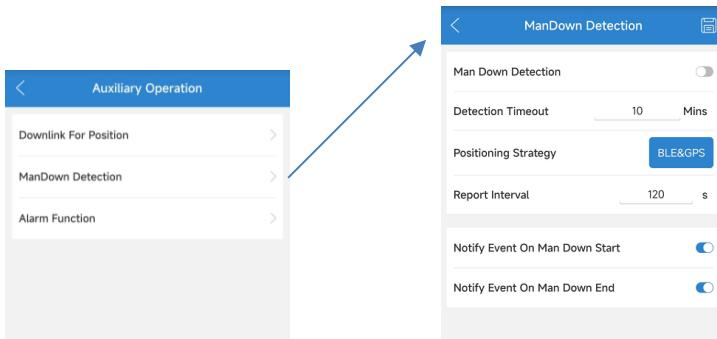
**Man Down Detection:** The function switch, the default is OFF.
