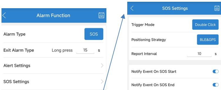
**Trigger Mode:** User can select the trigger way for SOS alarm. The default is double click.
