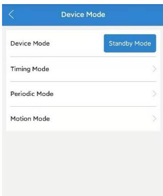
**Device Mode:** Users can choose different working modes according to different application scenarios. It can be set to standby mode, periodic mode, timing mode or motion mode. The default is periodic mode.
