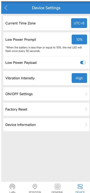
**Current Time Zone:** Selection of the time zone in which the current device is located.
