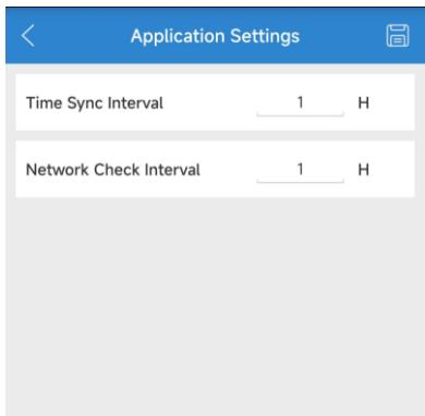
**Time Sync Interval:** It is used to sync the device time via MAC command. The default is 1, means that the device's time will be synchronized every 1 hour via LoRaWAN MAC commands.
