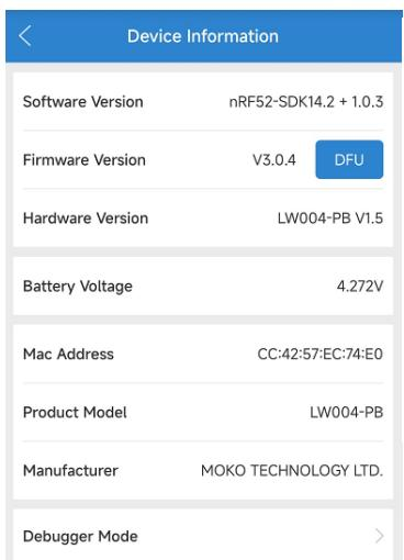
**Update Firmware (DFU):** To update the firmware via the DFU should use the upgrade package that MOKO provides with ZIP format. If you use an android phone, place the ZIP file of firmware upgrade package into the phone folder, select the upgrade package file from the OTA page of the APP, and click to upgrade.
