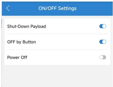
**Shut-Down Payload:** Whether to report shut-down payload. The default is ON.
