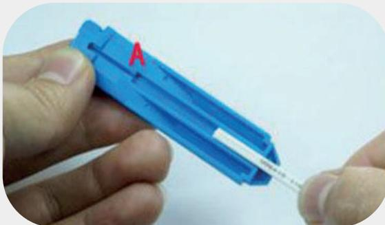
4. Peeled optical fibers, wiped with dust-free paper and alcohol.
