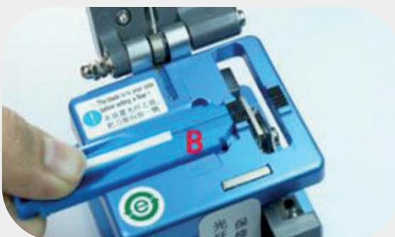
6. Use the cutting knife to complete the cutting.
