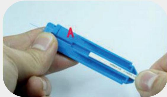
3. Pull the cable out and strip the coating.
