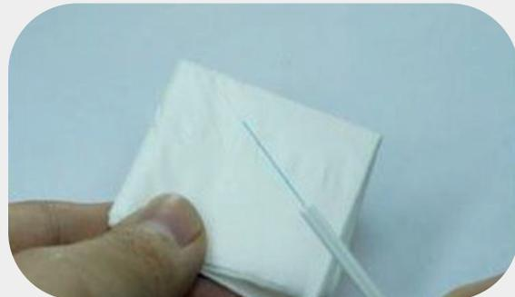
5. Optical fibers are placed on the fixed length surface and into the cutting tool chuck.
