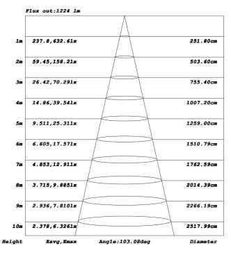
Remark: Above test data base on 18W 120Lm/W CCT 5000K @AC220V testing environment.
