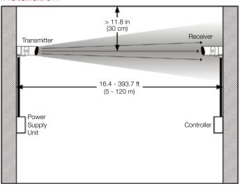
The distance between the ceiling and transmitter/receiver must be no more than 10 percent of the distance between floor and ceiling.
