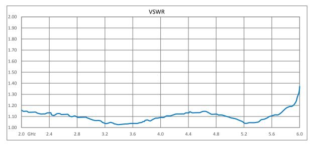
Click the following link (or enter part number in "SEARCH" on website) to obtain additional part information including price, inventory and certifications: Type N F/M Bulkhead Coaxial RF Surge Protector, 2GHz - 6GHz, DC Block, 10W, IP67, .5uJ, 10kA, Filter AL-LSXM-ME
