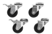
A set of four casters (two locking, two non-locking) that mount directly to the bottom of a ProLine frame, 0-mm or 100-mm Solid Base or a Console. (**Do not use on plinth bases**.) Casters elevate the enclosure 110 mm (4.33) when installed. Caster frames are plated steel with ball-bearing pivots. Caster wheels are made of a black polyamide material. Kit includes M12 mounting hardware.
