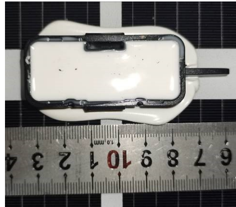
Junction box (opened)
