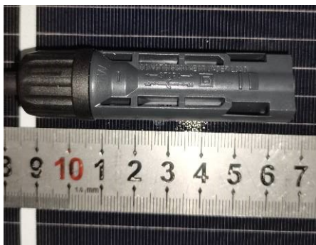
Mark (Do not disconnect under load)
