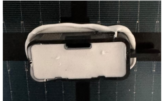
Junction box (opened)
