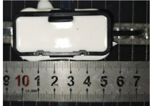
Junction box (opened)
