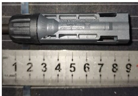
Mark (Do not disconnect under load)
