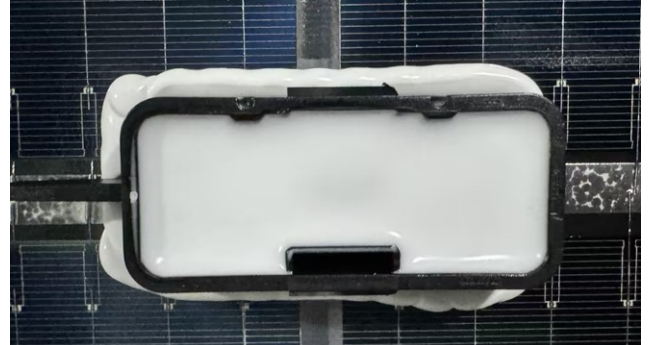
Junction box (opened)
