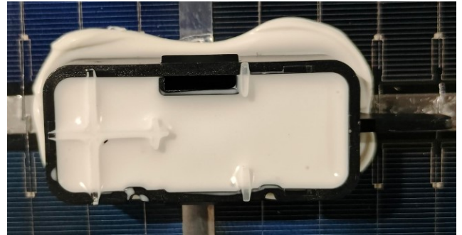
Junction box (opened)
